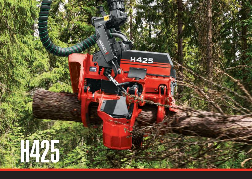
Optimizing performance, productivity and delimbing, the H425 excels in large diameter regeneration harvesting. With a powerful control valve and feed-roller arm geometry that ensures a solid grip, log control is only an afterthought.
